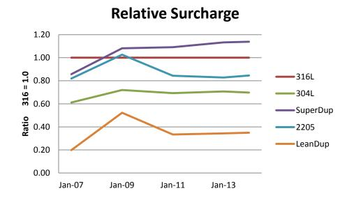
Figure 3b<sup>8,9</sup>: Relative Surcharge. Same as 3a except excluding the high nickel alloys.
